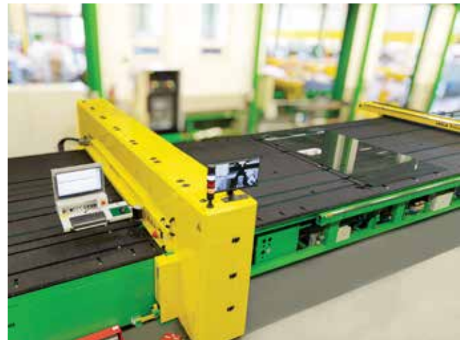
Fig. 1-3: The laser makes LSG cutting faster: throughput is increased by 20 percent or more, compared to conventional tube heating.
