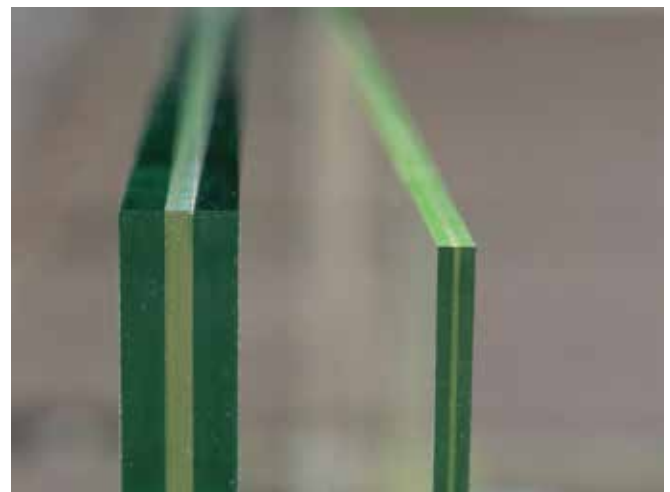
Fig. 4: The laser diode heater heats the scribe contour with pinpoint accuracy. The surrounding glass stays cold, thus preventing delamination at a later stage.
