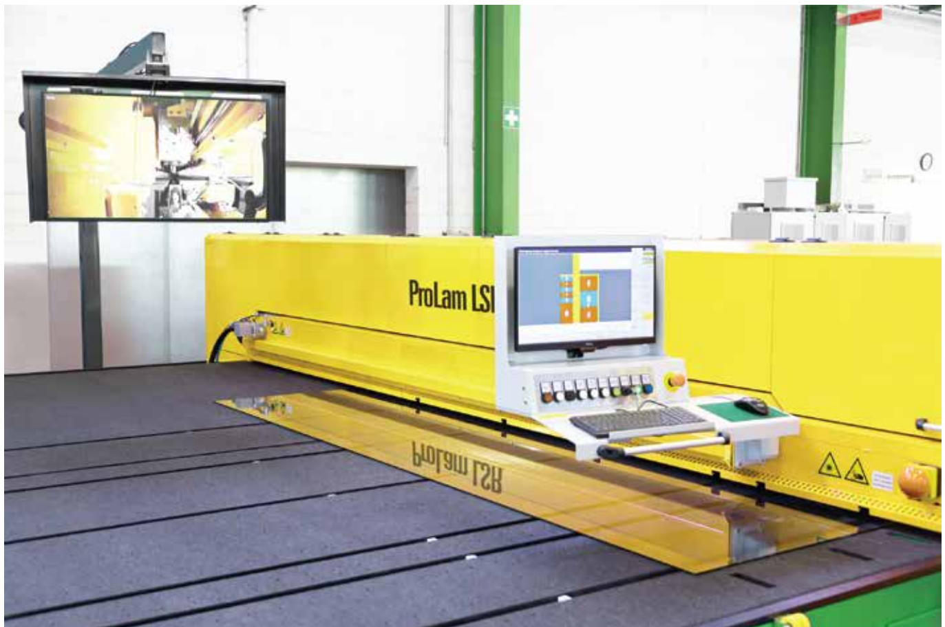
HEGLA is showing the ProLam LSR, a newly developed cutting system for LSG equipped for the first time with the time-saving laser diode heating technology as a system in series production. Up to 20 per cent and more productivity can be achieved with the new technology.
