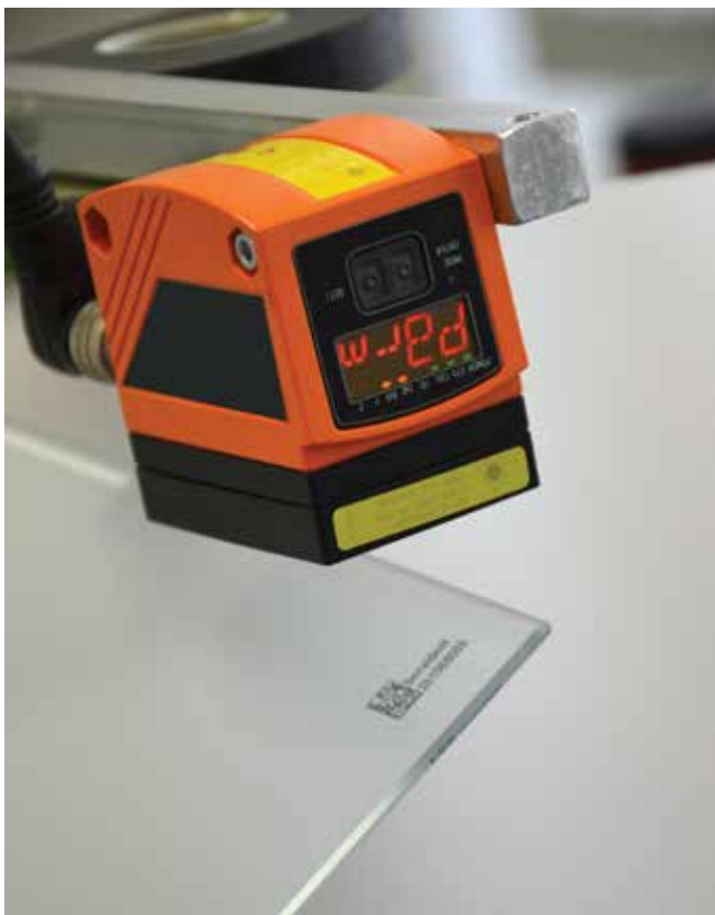
Track & trace is put into practice at HEGLA boraident. Via automatic scan or manually with an app, production progress can be recorded and tracked even years later.
