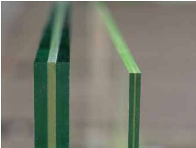
Demanding pane composites with up to ten-ply interlayer can be separated in a short cycle time with the new laser diode heating system. The precise application of heat to the cut contour means that the surrounding area virtually remains cold, preventing later delamination to the maximum extent possible.
