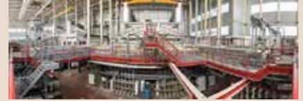
refractory and steel planning as well as its delivery, the combustion system, the tank and throat cooling, the measuring and control equipment, the boosting system, the reversing system, the stirring system, the HORN drainage system VARI-DRAIN® as well as the installation of the batch charging machine HVR® 700 S-2P.
