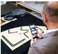
In cooperation with our partner Viprotron, A+W has developed a user-friendly, startlingly easy-to-use app to digitalize templates easily with a smartphone camera. Just fit the templates with L-shaped reference objects and then photograph them with a high-end smartphone camera. The reference objects, high-quality precision metal parts, are placed on the template or fastened to it. This corrects any distortions during photographing.
