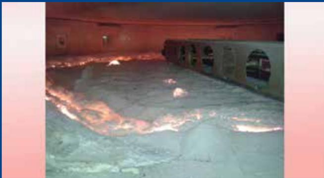
Cold batch on top of melt in full electric furnace.
