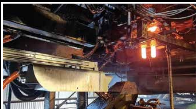
The Tiama HOT mass 2 provides glass manufacturers real 3D views of gobs and accurate measurements for gob shape such as length and diameters.
